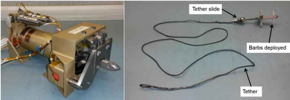
Figure 18. Harpoon firing device, projectile and tether.
