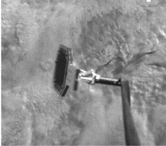
Figure 23. Target snapping off the end of the boom.
