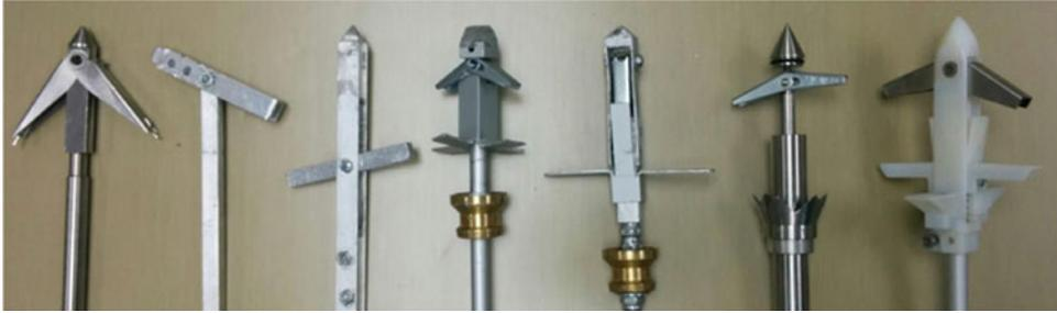
Figure 19. Harpoon tip and barbs design iteration.
