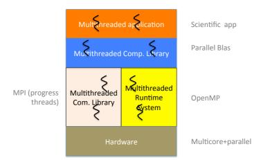
Figure 1: Software stack with different parts using threads
