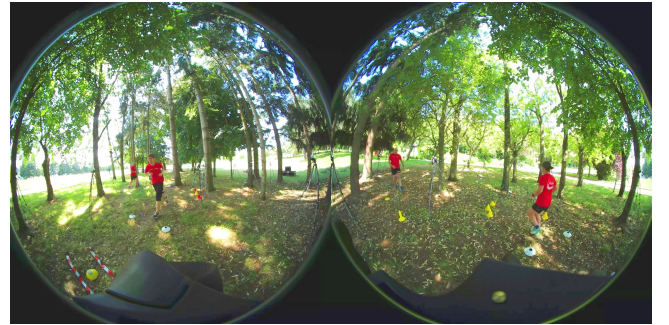
Figure 3: The used 360° cameras capture two hemispherical images leading to an image at a resolution of 3840 × 1920.
