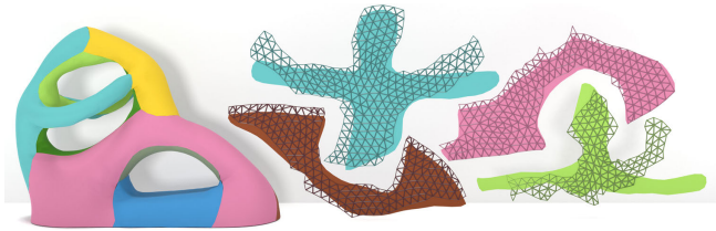
Fig. 14. Panel optimization. (Left) Optimized 3D shape. (Right) Comparison of the initial (wireframe) and the optimized (solid) 2D shape for a selection of panels.
