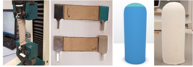
Fig. 12. Calibration process for measuring material parameters. (Left) Distances between reference points on strip samples are measured during uniaxial stretching to find Young's modulus and Poisson's ratio. (Right) Simulation and fabrication of a cylindrical formwork shape for validation.
