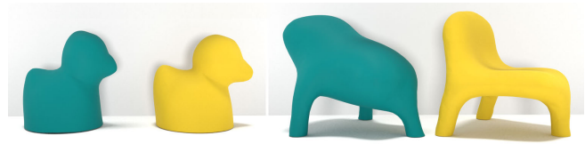
Fig. 5. Adding external supports can significantly improve the result of optimization. (Green) Optimized results without external supports, which are far different from the input models. (Yellow) Optimized results with support configuration as shown in Fig. 17.
