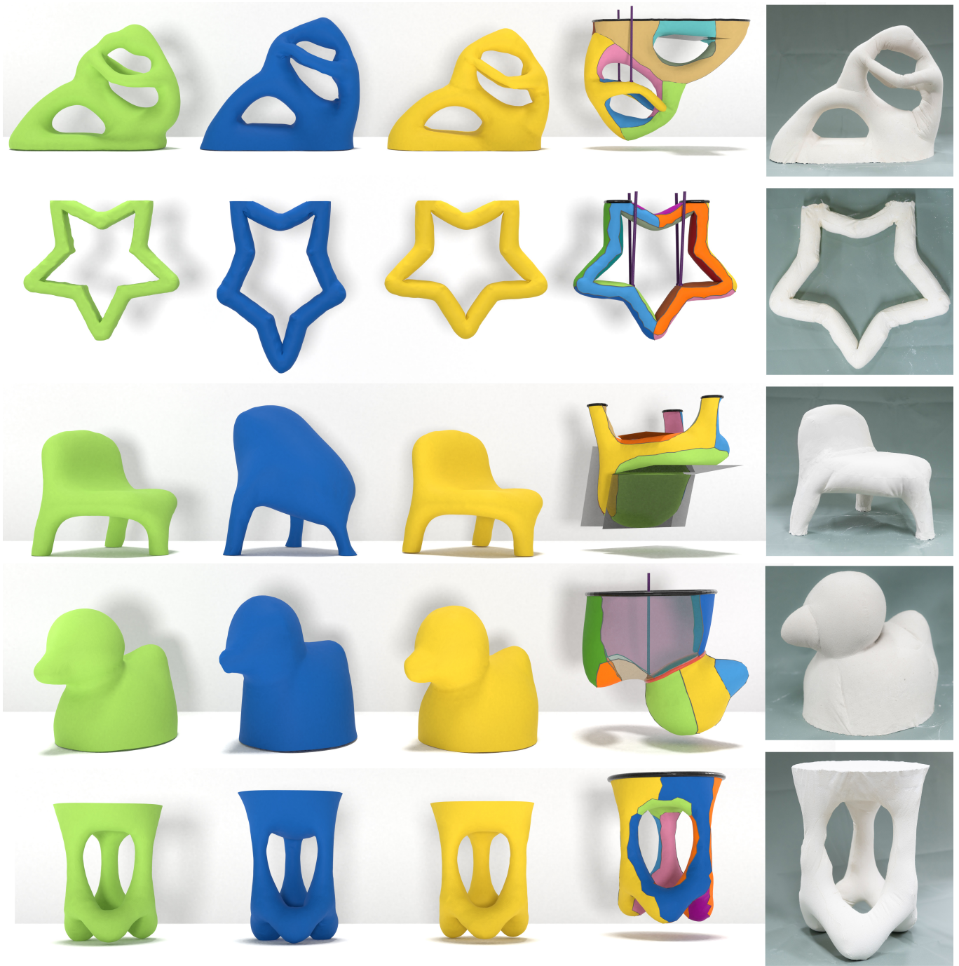
Fig. 17. Fabricated models. (Green) Target shape. (Blue) Deformed target shape simulated under force equilibrium (non-optimized panels). (Yellow) Optimized result: deformed shape with optimized panels, orientation, and external supports. (Inner-Right) Design configuration: colors correspond to individual panels, shown mapped onto the 3D shape. Gray lines indicate seams. Thick black lines along the top denote the suspension contact points. The fertility and star models both employ strings (dark purple lines). The chair uses four plane supports. The duck uses a string and a cable (red line) around the neck. A plane support is used for the table model under the green panel. Models shown in their optimized suspension orientation. (Right) Final plaster model resulting from the fabric formwork construction.
