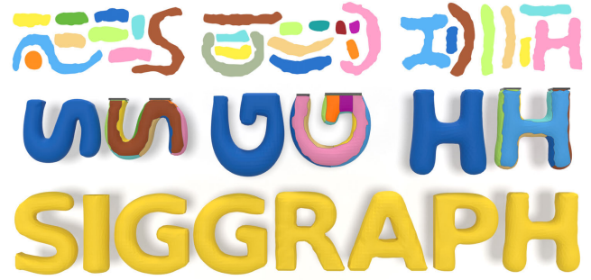
Fig. 7. Examples of optimized letter models. (Yellow) Optimized shape computed by our framework. (Blue) Deformed shape with unoptimized panels shown for comparison. (Multicolor) Design configuration with panels displayed in different colors and rotated according to fabrication orientation.
