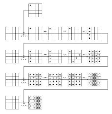
Figure 7: Integral distinguisher on 3 rounds of AES. A byte marked by 0 is balanced.
