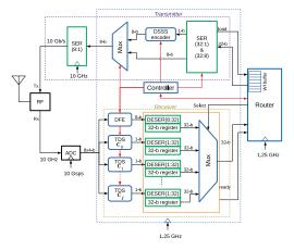
Fig. 3. Enhanced digital-domain transceiver architecture.
