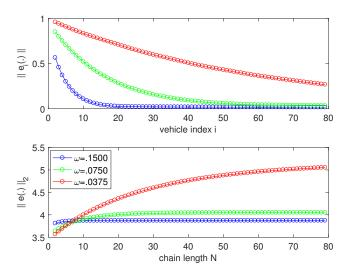
Fig. 5. Error  $\|e_i\|$  as a function of i (top) and  $\|e(.)\|_2$  as a function of N (bottom) for a disturbance input  $d_0(t) = \sin(\omega t)$  and three values of  $\omega$ .
