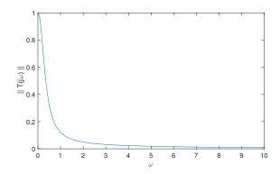
Fig. 2. Bode magnitude diagram of T(s) for the example of Section V. Note that we have avoided log-scales because it would squeeze the most important features, namely where  $||T(j\omega)|| \simeq 1$ .
