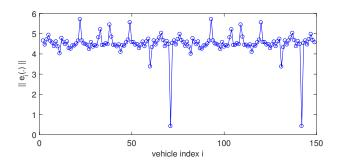
Fig. 3.  $\|e_i\|$  as a function of i when  $L_2$ -norm bounded disturbances are applied on all the vehicles. The  $(L_2,\ell_\infty)$  string stability criterion for chain length N is given by  $\|e(.)\|_\infty = \max_{i \leq N} (\|e_i(.)\|)$ ; it remains bounded  $\|e(.)\|_\infty < 6$  for any N.
