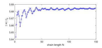
Fig. 4. Error  $(L_2,\ell_2)$ -norm  $\|e(.)\|_2$  as a function of N when the same disturbances are applied as on Fig.3, up to rescaling such that  $\|d(.)\|_2 < 1$ . This curve appears to saturate at large N.
