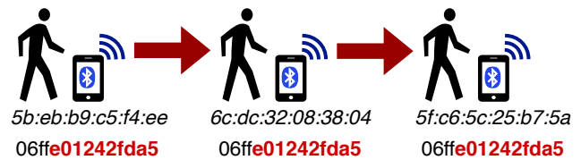
Figure 5: Representation of a successful attack. The BLE device is randomizing its BD_ADDR (in italic) over time while keeping a static identifier (in bold) in the advertising data. Such a 5-byte identifier can be used by a passive attacker to link together the packets generated with the three different BD_ADDR.
