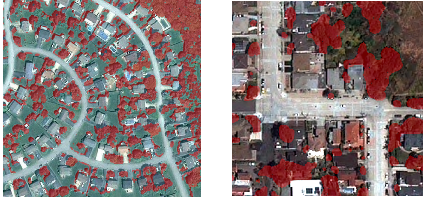
(a) Pittsburgh (b) San Diego Figure 2: Example of available imperfect ground truth for trees.
