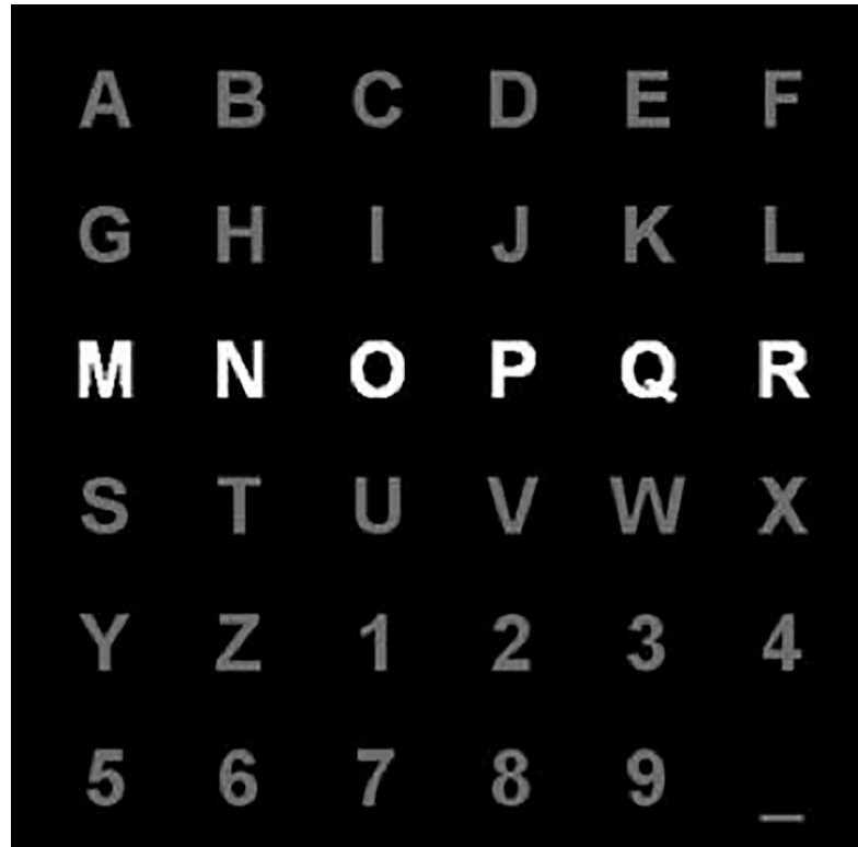
Fig 3. A matrix which contains letters of the alphabet and other symbols, which are flashed in random order (white line on the image) to elicit the P300 evoked response based on [35].
