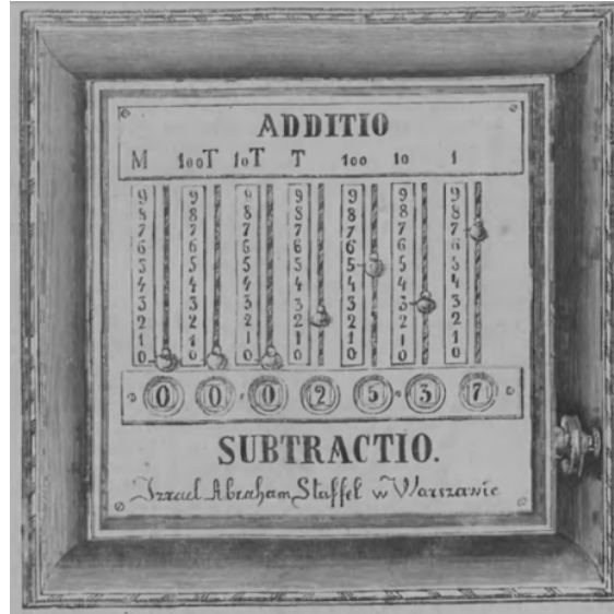
Fig. 4. Staffel's adding machine of 1858 [11].
