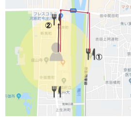
Fig. 2. Difference of the Euclidean distance and the shortest path length on a road network.
