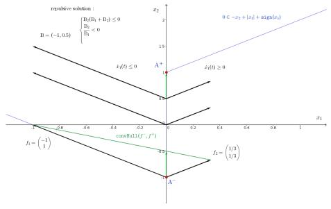
(b) Example of solution with B=(-1,0.5) which corresponds to repulsive solutions along the switching surface. The vector field of the reduced system is in black, and its convex hull is given in green.
