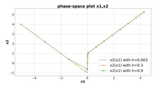
Fig. 5: Phase space plot in  $(x_1, x_2)$  of the numerical solutions for the sliding crossing case,  $B = (-0.5, 1)^T$ , and h = 0.9, h = 0.3, or h = 0.003. Initial condition is  $\mathbf{x}_0 = (-5, 4)^T$ .
