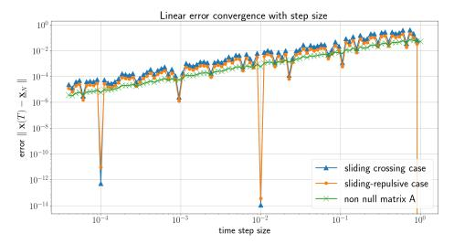
Fig. 7: Error  $\|\mathbf{x}(t) - \underline{\mathbf{x}}_N\|$  with respect to time step h. We consider the two kind of AC solutions: the sliding-crossing solutions and the sliding-repulsive solutions.
