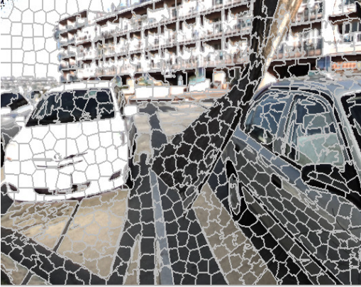
Fig. 1: An example of super-pixel segmentation for the Cars dataset, obtained by fixing the number of superpixels to 800.
