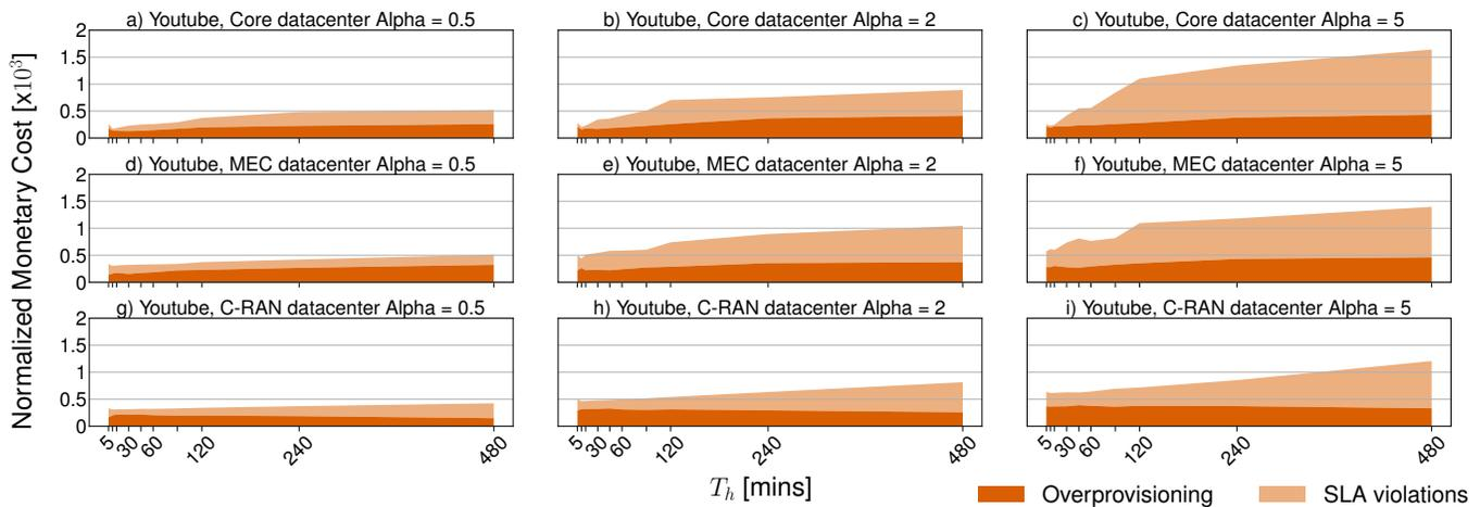
Fig. 9. Monetary cost (normalized by the cost of one capacity unit) incurred by the operator, versus the prediction time horizon  $T_h$ . The plots refer to different combinations of datacenter class and economic strategies modeled by  $\alpha$ , for a slice dedicated to the YouTube mobile service.
