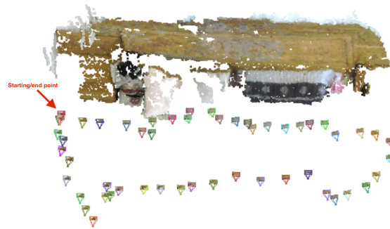
Figure 8. Structure from motion test. Top: Panorama stitched by Hugin ( http://hugin.sourceforge.net ), showing the test scene. Bottom: Result of applying VisualSfM [22] to build a 3D model. We started capturing images from the left and moved clockwise, finally came back approximately to the starting point.
