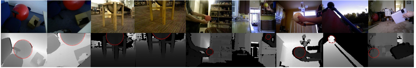
Figure 12. Qualitative visualizations of sphere detection in the wild: Our algorithm successfully detects primitives in difficult scenarios including clutter, occlusions and large distances. Note that the sphere is detected in 3D only using the point clouds of depth images and we draw the apparent contour of the quadric. The RGB pictures are also included in the top row to ease the visual perception.
