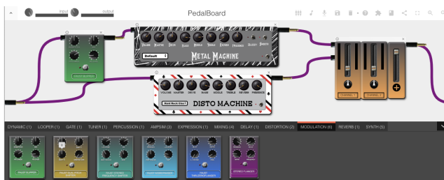
Figure 1: the virtual pedalboard host application scans multiple remote WAP plugin servers. WAP plugins can then be dragged and dropped and assembled in a graph.
