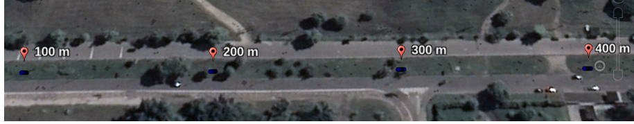
Figure 11: CooPS absolute position validation. The landmarks 100, 200, 300 and 400 m are the corresponding ground positions from RSU_A . The errors are acquired from the comparison between CooPS estimation positions and Google Earth map positions (figure produced using Google Earth).
