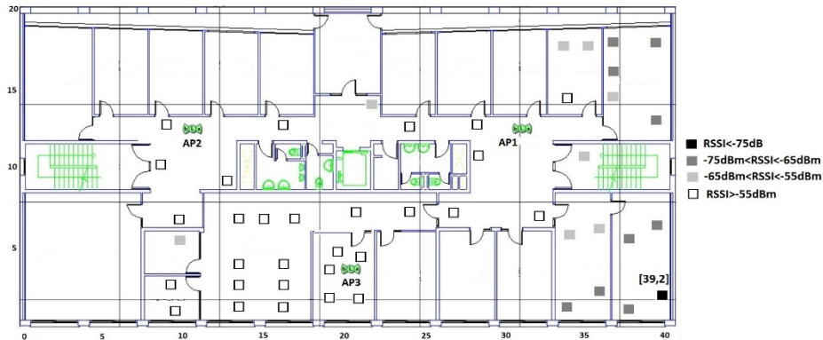
Fig. 4. RSSI measurements obtained before the AP Relocation i.e. AP3 at [20,4] .
