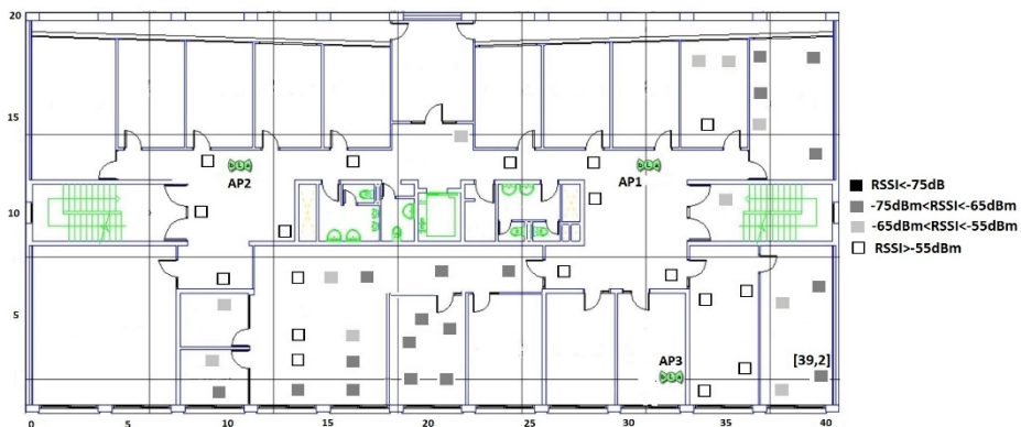
Fig. 5. RSSI measurements obtained after the AP Relocation i.e. AP3 at [32,2] .
