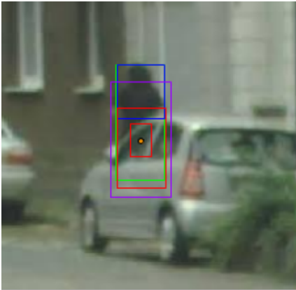
Figure 6. An occluded pedestrian with full-body bounding box ( green ) and visible bounding box ( blue ). Red anchors are confocal with the magenta anchor. The red anchors do not overlap well with both the full-body and visible bounding box, while the magenta anchor has sufficient overlap with both.
