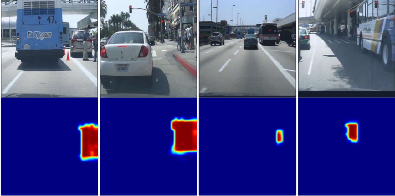
Figure 4. (Top: Original images. bottom: O_{cp} from spatial attention. O_{cp} has been resized to original image size with bilinear interpolation for better visibility.
