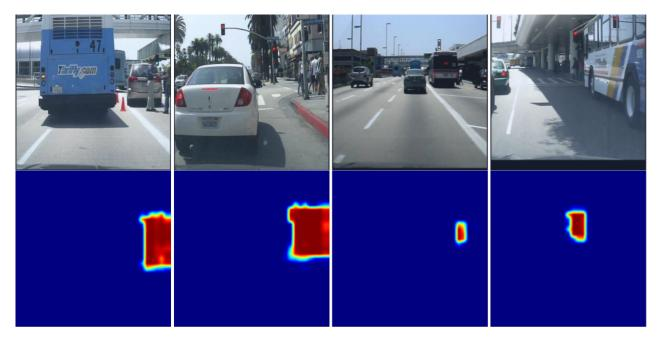
Figure 4. (**Top**: Original images. **bottom**:  $O_{cp}$  from spatial attention.  $O_{cp}$  has been resized to original image size with bilinear interpolation for better visibility.
