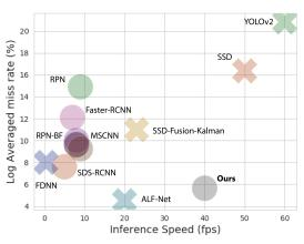
Figure 1. Speed/Accuracy scatter plot of various pedestrian detectors categorized into one-stage(crossed) and two-stage (circles) detectors for the caltech-reasonable testing set dataset.
