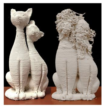
Fig. 8. The Two Cats model printed using our continuous deposition method (left) and the reference slicer (right).
