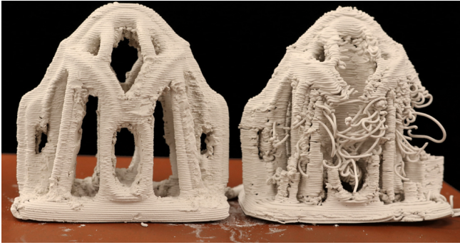
Fig. 7. The Spire model with multiple disconnected components printed using the reference slicer ( right ) and our method ( left ).
