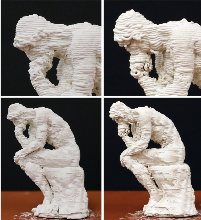
Fig. 9. Comparison between our continuous deposition method ( left ) and the reference slicer ( right ) on the Rodin model. The reference slicer produces severe defects around the wrist ( top right ) and ribs, as well as many over-extrusion artifacts. Our method produces an intact wrist ( top left ) and generally cleaner layer structure with much fewer artifacts.
