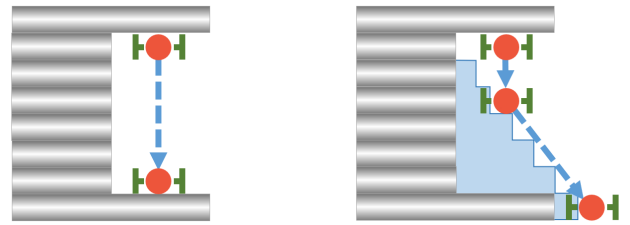
Fig. 4. Side view of safeguard. Left : generating paths from top to bottom, the non-model structure (red) cannot be displaced enough to avoid the model (grey) once the collision is detected. Right : using the safeguard (blue), our algorithm can anticipate the collision with model and exploit the admissible horizontal offset (green) to displace the non-model structure early enough to avoid collisions.
