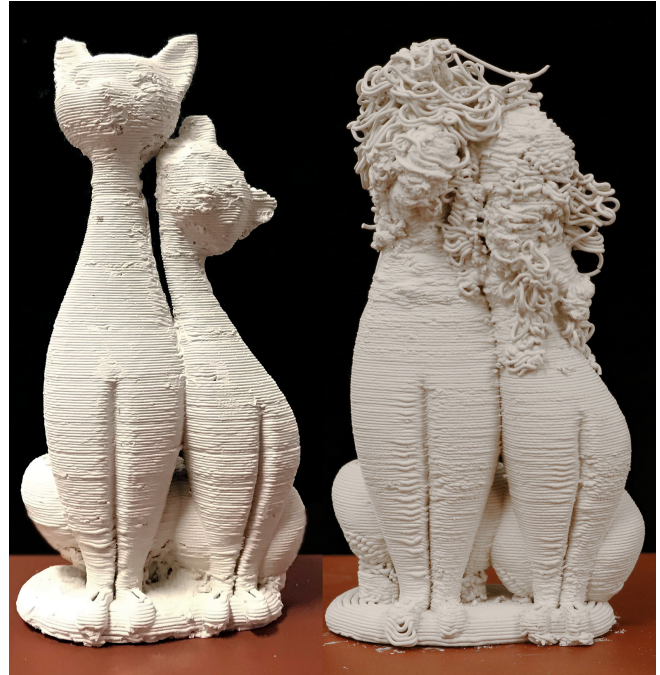
Fig. 8. The Two Cats model printed using our continuous deposition method ( left ) and the reference slicer ( right ).
