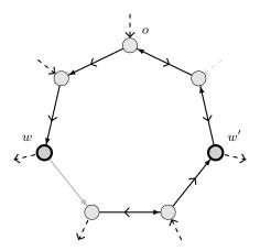
FIGURE 2. Flow directions and resulting flow-meeting points. Bold arcs indicate entry-exit activity and flow directions, whereas gray arcs indicate inactive nodes or zero arc-flow. In this example, exits w and w' are flow-meeting points.
