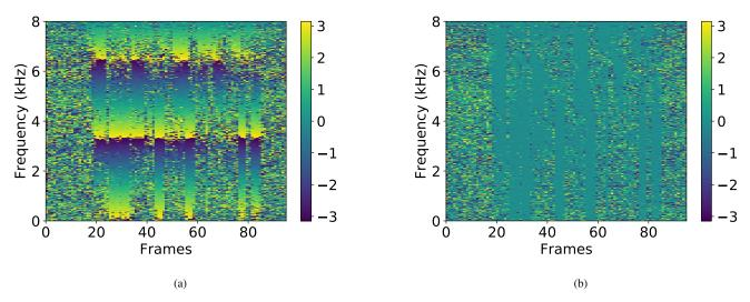
Fig. 2: Phase difference in presence of noise before DS beamforming (2a) and after DS beamforming (2b)
