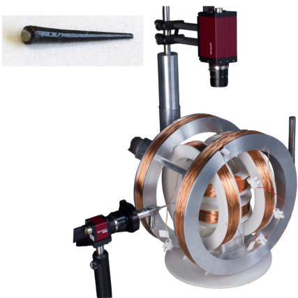
FIG. 1. Experimental setup ([21]). The three orthogonal Helmholtz coils generate a homogeneous magnetic field in the center, where the swimmer has been placed. The swimmer is tracked using two perpendicular cameras. In the corner: Scaled-up flexible magnetic swimmer used in the experiments.
