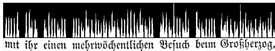
Fig. 2. Original text line and its vertical projection profile.
