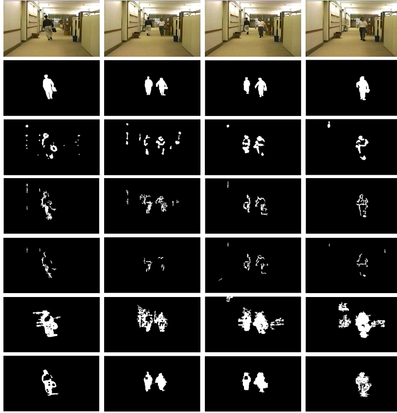
Fig. 2: Results with Video 1 for the frames number (a) 72 th (b) 191 th (c) 222 th (d) 265 th ; row wise, up to down: original frame, ground truth, Sukumaran [33], Fei [3], Yin [34], Sengar [5], and the proposed method.
