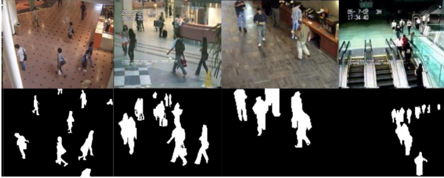
Fig. 2. Results of foreground/background subtraction (pictures in second row represent extracted foreground objects)
