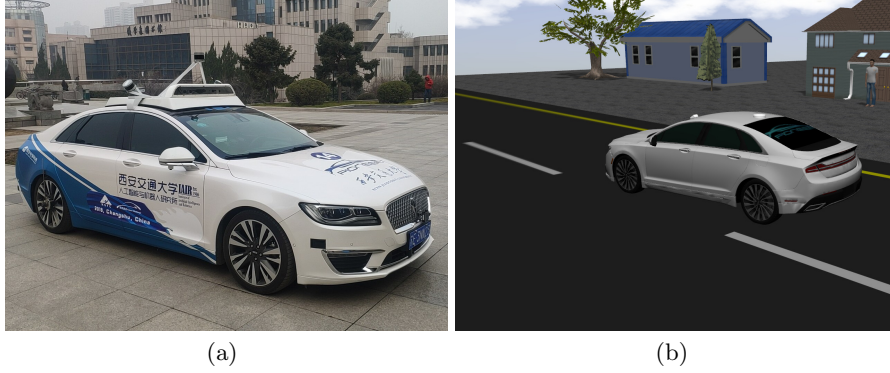
Fig. 4. (a) The self-driving experimental platform “Pioneer”, based on 2017 Lincoln MKZ hybrid model. (b) The simulation platform based on Gazebo. Various experimental scenarios can be built in this simulation platform.
