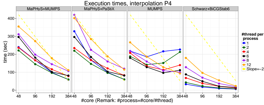
FIGURE 2 Plane wave propagation in vacuum: Strong scalability analysis of simulations run on the Plafrim cluster. On each plot, the various figures correspond to different configuration of subdomain partitioning (MPI parallelization) and threads within each subdomain.
