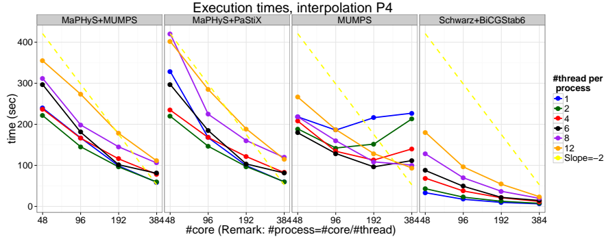
FIGURE 2 Plane wave propagation in vacuum: Strong scalability analysis of simulations run on the Plafrim cluster. On each plot, the various figures correspond to different configuration of subdomain partitioning (MPI parallelization) and threads within each subdomain.
