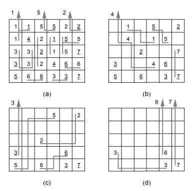
**Fig. 6.** (a) Layer 1 with the first connections. (b) Layer 2. (c) Layer 3. (d) Layer 4. Arrows indicate the connections to the input leads on the top edge. Underlined literals indicate the starting cells of the vias.
