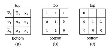
**Fig. 1.** A network of four terminal switches implementing the function  $f = x_1x_2x_3 + \overline{x_1}\overline{x_3} + \overline{x_2}\overline{x_3}$  (a); the lattice evaluated on the assignments 1,0,0 (b) and 1, 0, 1 (c), with 1's and 0's representing ON and OFF switches, respectively.
