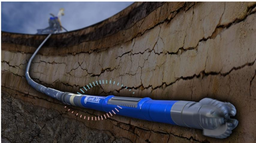
Guide the drilling trajectory using “real-time” magnetic measurements
