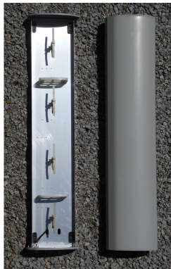
Figure 20: Interior of sector antenna (MIT Computer Science & Artificial Intelligence Lab). An array of dipole antennas in a "+" configuration to transmit the same signal on two perpendicular polarizations in order to minimize polarization mismatch at reception. Hence, improves cellular reception.
