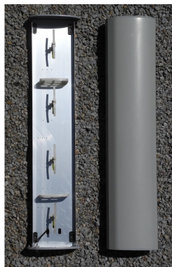
Figure 19: Interior of sector antenna (MIT Computer Science & Artificial Intelligence Lab). An array of dipole antennas in a "+" configuration to transmit the same signal on two perpendicular polarizations in order to minimize polarization mismatch at reception. Hence, improves cellular reception.
