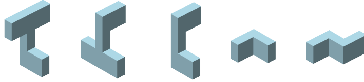
Fig. 9. Typical, pre-defined wiring and via patterns that have to be simulated by FEM in addition to those from Fig. 6.
