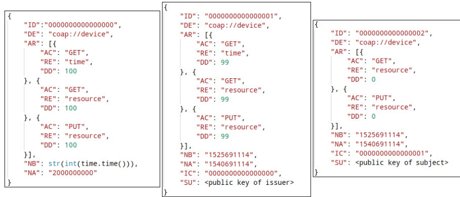
Fig. 6. An example of a delegation chain showing the JSONs used during the issuing of the respective capability tokens. The leftmost one is for a root capability. Following the same delegation relations shown in Fig.1, both 1st and 2nd capabilities (from the right) are issued by the device , while the 3rd one by the issuer .
