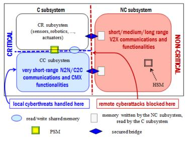
Fig. 1. Schematic architecture of a NGV onboard system
