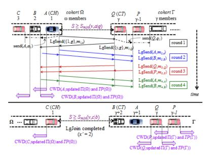
Fig. 9. Illustration of a LgJoin cyberphysical operation
