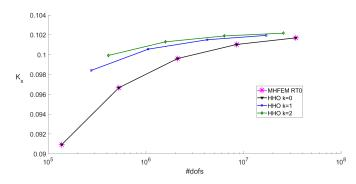
Figure 3: Test case B0: x-component of the equivalent permeability tensor.
