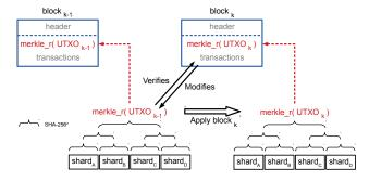
**Figure 2:** The UTXO set is updated at every block validation. For a counterfeited block to be validated by diet nodes, a malicious miner has to forge at least two consecutive blocks: the first block  $B_{k-1}$  containing a fake UTXO Merkle root of UTXO<sub>k-1</sub>, and the second block  $B_k$  spending fake coins validated by the fake UTXO<sub>k-1</sub>.
