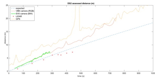
Fig. 18: Tracking results synthesis: DSAT2 assessed distance (expected distance in blue).
