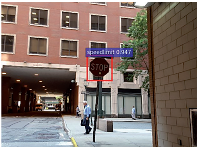
Figure 45: Putting a small, innocent-looking sticker on a STOP-sign can make it look like a speed limit sign to a machine learning algorithm trained to (un) correctly classify (US) street signs. Source: [203]
