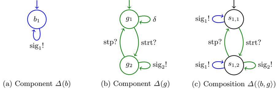
Figure 1: A simple component-based sensor node example.
