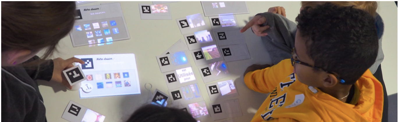
Figure 1. CARDS is a Mixed-Reality system targeted at Education where both physical and digital content are manipulated by several users in a seamless workspace.
