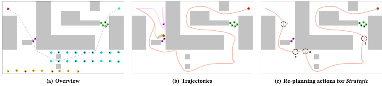
Figure 6: Single-agent demonstration. (a) An agent is instructed to move from the top left to the top right. The curve is its initial global path. (b) The agent’s trajectory using CA-Only (pink), Standard (brown), and Strategic (red, with T_R = 2 , W = \infty , and Strict = False). (c) The Strategic agent changes its global path on several occasions, indicated by the black circles.
