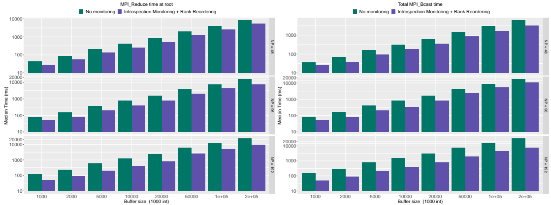
(a) MPI_Reduce (MPI_MAX) walltime (x and y log-scale) for 48, 96 and 192 ranks and various buffer sizes. Binary Tree algorithm. (b) MPI_Bcast walltime (x and y log-scale) for 48, 96 and 192 ranks and various buffer sizes. Binomial Tree algorithm.
